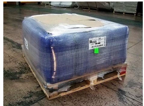
Drums, tied down and properly wrapped
