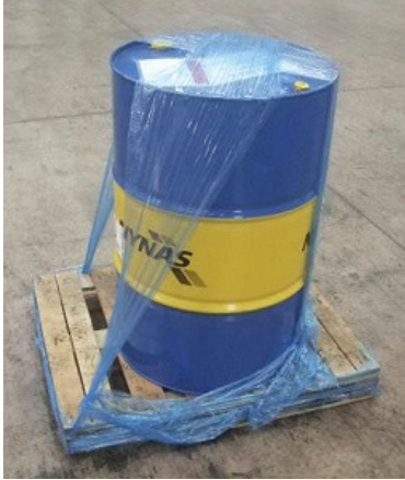
This drum is barely secured.
