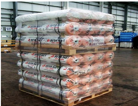
Rolls, stacked, supported, and shrink wrapped
